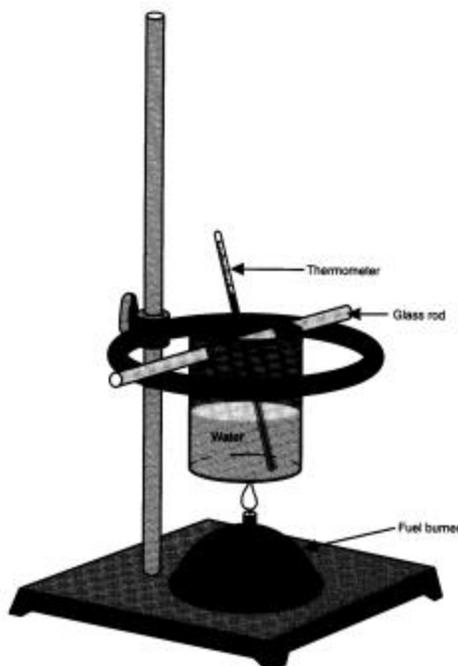
Diagram of can and burner setup
